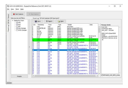
The AUX Analyzer tabs collect AUX Channel Transactions from the Event Log in the *Transaction list*. The user can parse the content of each transaction by clicking the corresponding *transaction line*. The parsed content is in the *Message Details* panel on the right.
