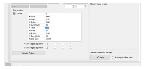
The timing parameters can be modified by selecting the **Custom** check-box and editing the fields of the matrix. Enable the new parameters by clicking **Apply** button.
