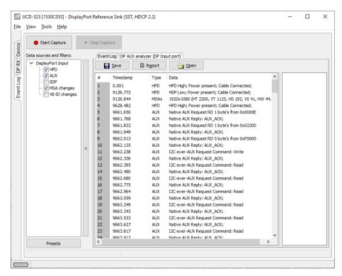
Event Log dialog is divided into three panels: *Data sources and filters* panel on the left enables selection of the items to be logged. The selection of data sources is dependent on the role selected: DP Input, DP Output, HDMI Input, HDMI Output.
