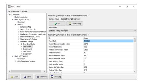
The *EDID Editor* main window is divided into three logical areas. The bottom part of the window contains the command buttons, and the log view. The top-left portion shows the currently edited E-EDID blocks in a tree-form, and the top-right portion shows an edit control for the currently selected item, possibly a list of sub-keys and their names (The list is not shown for all values) and the HEX-view of the block collection.
