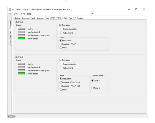
HDCP tab is the dialog for monitoring the HDCP (for *High-Bandwith Digital Content Protection*) status and controlling the HDCP capabilities of the connected UCD-300 device.
