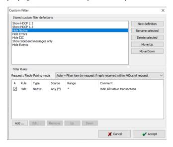
In the *Stored custom filter definitions* panel, lists currently defined Filters. On the right hand side buttons, you can define new Filters, rename or delete them. Their appearance in the *Filters* pull-down menu can also be altered.
