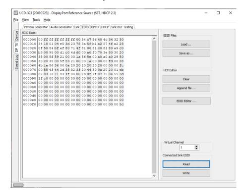
EDID tab will enable analyzing and saving the EDID read from the connected Sink device.
