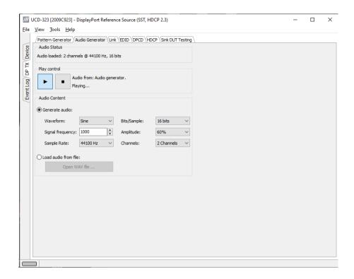
Audio generator allows the user to play LPCM audio generated internally or from files in WAV format.
