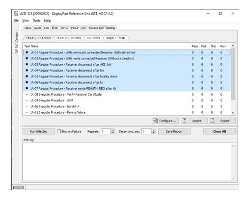
**Repeats** defines number of test-runs and the **Delay time** delay between the tests. When repeating a sequence of tests, all selected tests are performed in each repetition. E.g. when you repeat tests 1, 2 and 3 two times, the sequence is: 1, 2, 3, 1, 2, 3.
