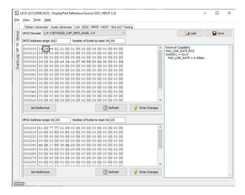
DPCD tab is a tool for monitoring and editing the DPCD registers of the connected Downstream Sink.
