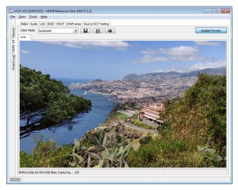
The measured input resolution, frame rate and color format is shown below the preview window. The indication of the number of frames captured to the PC shows you the pace of the image data transfer to the PC.
