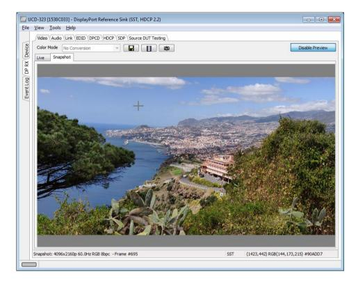
**Color Information of the Captured Bitmap** can be evaluated by placing the mouse cursor on top of the preview image. The lower right-hand side ribbon of the GUI lists
