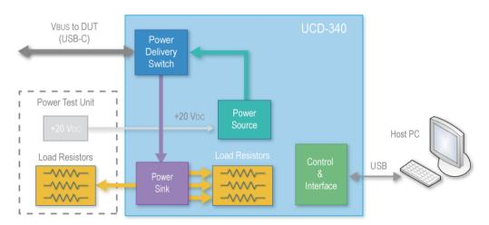
Please find below a matrix describing Power Source and Power Sink options of UCD-340 internally and with attached *Unigraf External Power Test Unit*. Please find description of controlling the power options with UCD Console later in this manual.
