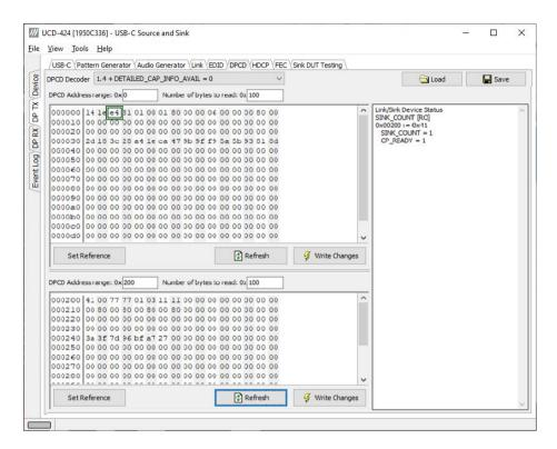
The tool consists of two independent monitoring and editing windows for the DPCD data. The user can freely select the the DPCD address areas shown on each panel.
