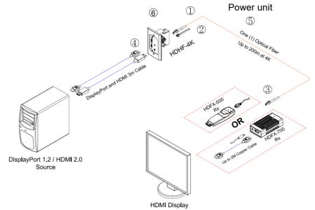
1 Connect Power cables into 3-pin power connector of HDHF-4K.
