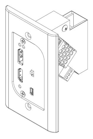
HDMI 2.0 and DisplayPort 1.2 to HDMI 2.0 optical converter, HDHF-4K
