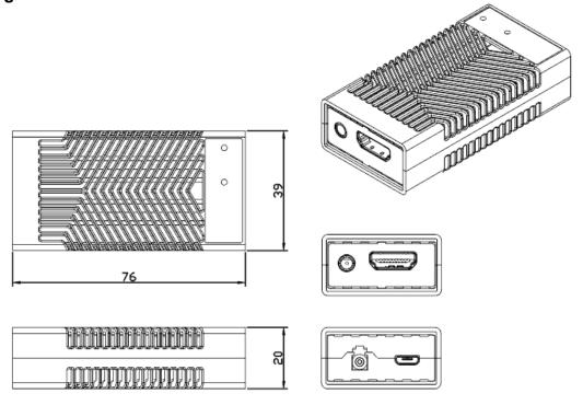
Note: The transmitter, HDFX-700-Tx and the receiver, HDFX-700-Rx have the same mechanical dimensions
