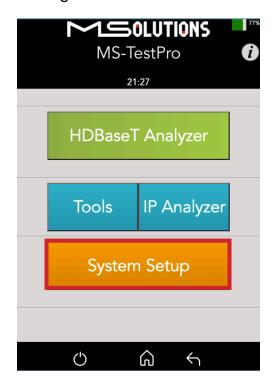
The image adjacent is for the legacy GUI of the MS-TestPro. To find the current firmware version, click 'System Setup'.
