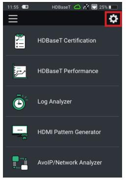
The image adjacent is for the new GUI of the MS-TestPro. To find the current firmware version, click the 'Settings' icon in the top right of the Home screen.'
