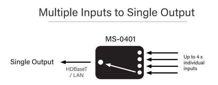
The MS-0401 can also be used to route any of up to 4 x input signals to the output.
