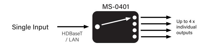
The MS-0401 can be used to transfer the signal from one point of transmission to one of the 4 x outputs. When there is no power to the MS-0401, port 1 is automatically selected as a static pass-through.
