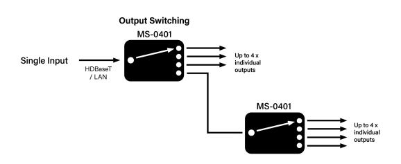
Networks and HDBaseT connectivity can be expanded using multiple MS-0401 units inline between point of transmission to receive. Adding in a subsequent MS-0401 unit will provide connectivity to up to 7 x displays from a single source. Cascading can also work for extra inputs.
